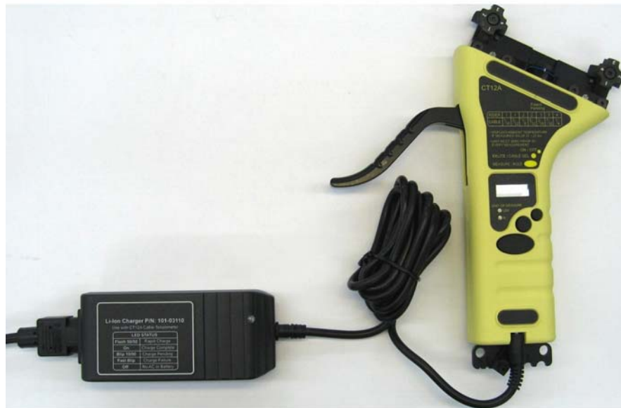
Figure 8 CT12A with Battery Charger Accessory
