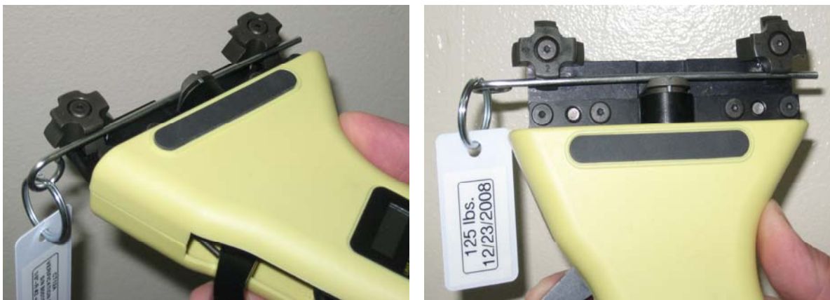
Figure 7: Two views of the correct placement of the Verification Bar in the CT12A
