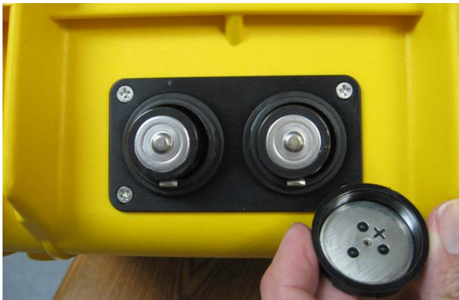
Figure 7 CORRECT BATTERIES POSITION
